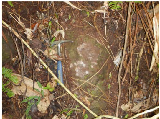
Photo 3-35: Outcrop of Andesite classified as CM Class Rock at Right Bank along Proposed Headrace
