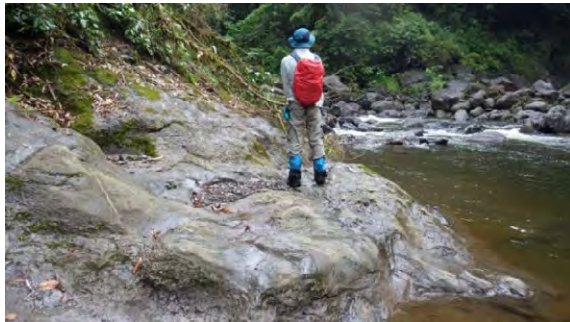
Photo 3-22: Outcrop of the Andesite classified as CH Class Rock at the Right Bank of Proposed Intake Weir Location
