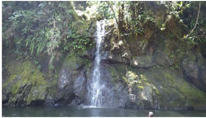
Photo 3-31: Water Fall and Andesite Outcrop classified as CM Class Rock at Left Bank along Proposed Headrace
