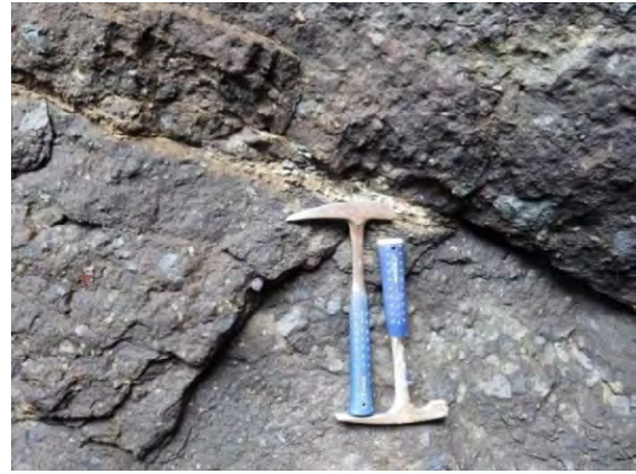
Photo 3-17: Close up of the Photo-24. Discontinuities show Strike of 62 Degrees North-East Direction and Dip of 32 Degrees Southeastward
