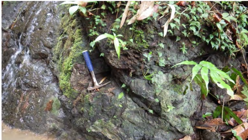
Photo 3-3: Andesitic Tuff Classified as CL to CM Class Rock at the Right Bank of Location Proposed Intake Weir
