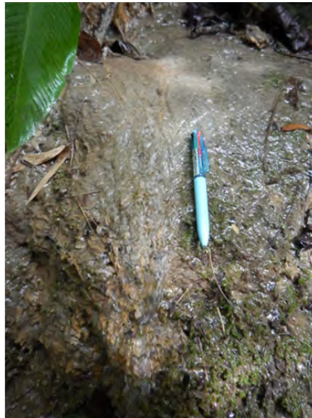
Photo 3-12: Outcrop of Dissolute Limestone classified as D Class Rock at Right Bank along Route of Proposed Headrace
