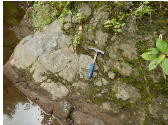
Photo 3-39: Outcrop of Andesitic Tuff Breccia classified as CM Class Rock at Right Bank of Proposed Power House Location
