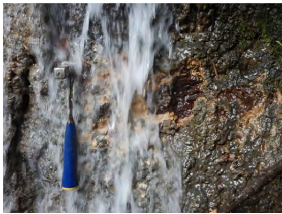
Photo 3-4: Boundary of Limestone and Tuff at the Right Bank of Location Proposed Intake Weir
