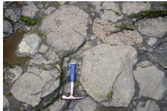
Photo 3-19: Andesite with Columnar Joints classified as CM Class Rock on Riverbed.
