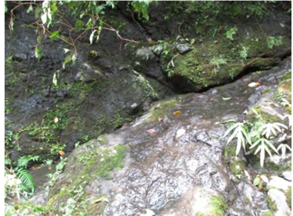
Photo 3-30: The Boundary of Andesite and Andesitic Tuff
