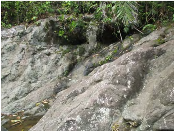
Photo 3-6: Andesitic Breccia classified as CM Class Rock at the Left Bank of Location Proposed Intake Weir
