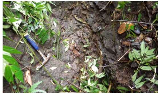
Photo 3-28: Outcrop of Andesite classified as CM Class Rock
