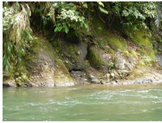
Photo 3-7: Andesitic Breccia classified as CL Class Rock at the Left Bank of Location Proposed Intake Weir
