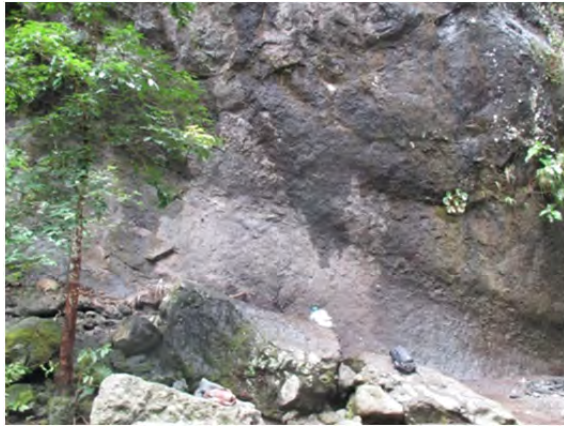
Photo 3-16: Andesitic Tuff Breccia classified as CL Class Rock exposed at Surface of Cliff at the Right Bank of Location Proposed Intake Weir on Wawa River
